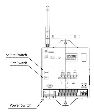
Turn on the power switch while pressing SET key to start mode setting.
