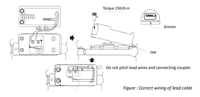
Please perform transmitting test after finishing. If transmission error happens during test, make sure LS switch position is correct. Check LS lever switch position when torque wrench clicks. If further problem, contact Tohnichi.
