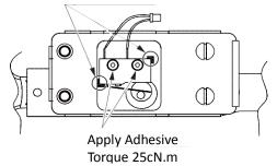
Set attached LS switch on the predetermined position. Apply adhesive and tighten with 25cN.m. There is a tiny washer for each screw.
