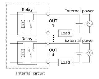
Set the load of the contact output within the rated load. Relay output rating: DC30V 1A, AC125V 0.5A. The above rated contact capacity is according to resistance load. Some kinds of loads have a big difference between the steady-state current and the inrush current. Typical loads and inrush currents are as follows:
